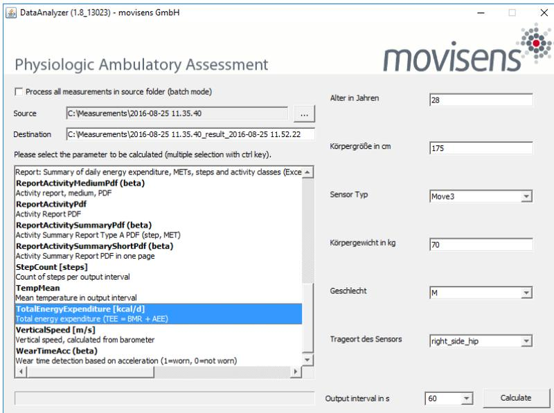
After selecting a measurement, the **DataAnalyzer** displays all the possible analysis outputs (secondary parameter and reports). The list of analysis outputs depends on your licensed modules and the data contained in your measurement. You can now select the desired
