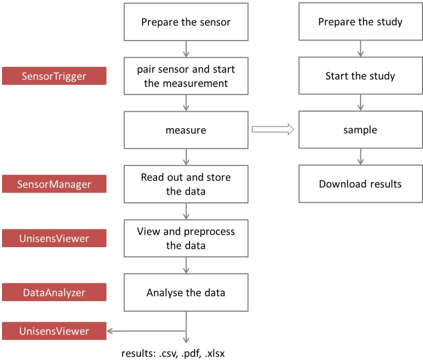
The right side of the diagram illustrates the process to prepare and run a study on **movisensXS**.
