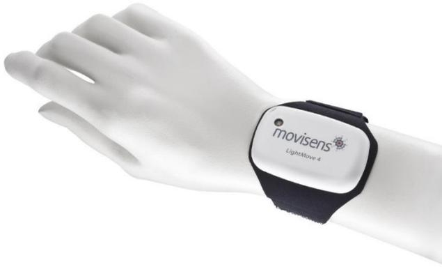
**LightMove 4** is also equipped with a Bluetooth Smart interface. The sensor can be used in conjunction with a gateway or a mobile phone for live applications. The Bluetooth Smart interface is activated in the default configuration of the sensor. To deactivate this interface, a firmware update is required (see 6.4)
