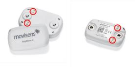
✓ After connecting the sensor to a USB port, the charging process starts immediately. During charging, the status LED is blinking blue. If the sensor is fully charged, the LED is blinking green. The charging process of the sensor can take up to two hours, depending on the battery status of your sensor.
