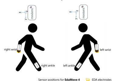
**Step 1:** Connect the **EdaMove 4** sensor to the wrist strap and lay the sensor on a flat surface in front of the test subject. Make sure that the electrode cables are lying towards the subjects elbow, not the fingers and ensure that they are separated on either side of the arm.
