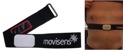
Fig. 1. The Movisens sensor and the sensor belt: On the inside of the sensor belt one of the two dry electrodes is visible.
